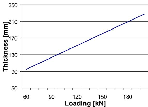
Fig. 6 Design diagram: Thickness vs. Point loading Intensity of a back to back leg case.
