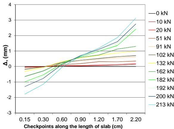
Fig. 5 Deflections recorded from 0.3 m distance to 2.20 m distance.
