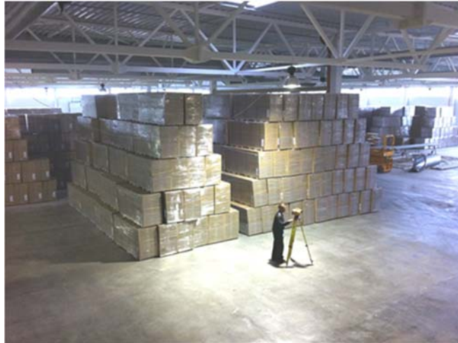
Figure 7: Full scale loading test of the Klaipeda (Lithuania, 2011) PrimeComposite slab-on-piles.
