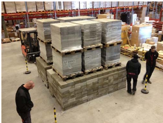
Figure 8: Full scale loading test of the Tingstad project (Gothenburg, Sweden, 2014) PrimeComposite slab-on-piles.
